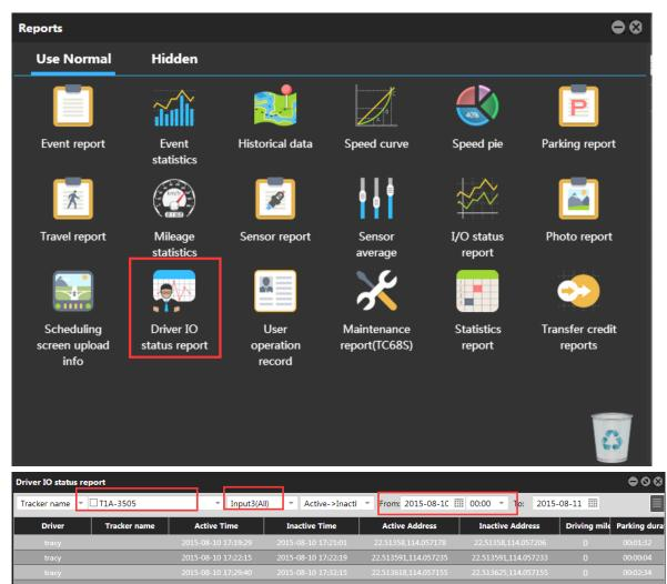
Note: In this report, input 3 is connected to the engine detection cable. You can obtain the driver's driving duration, mileage,
